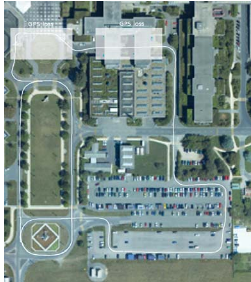
Fig 9: Overlay of the filtered trajectory on the ortho photo of the EPFL campus.
