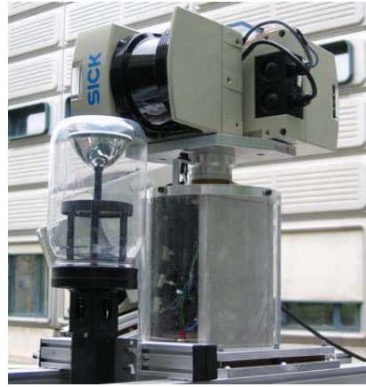
Fig 4: Omnidirectional camera and rotating sick
