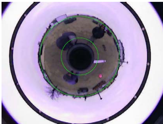
Fig. 17: The omnidirectional picture of the road, with isolated region of interest
